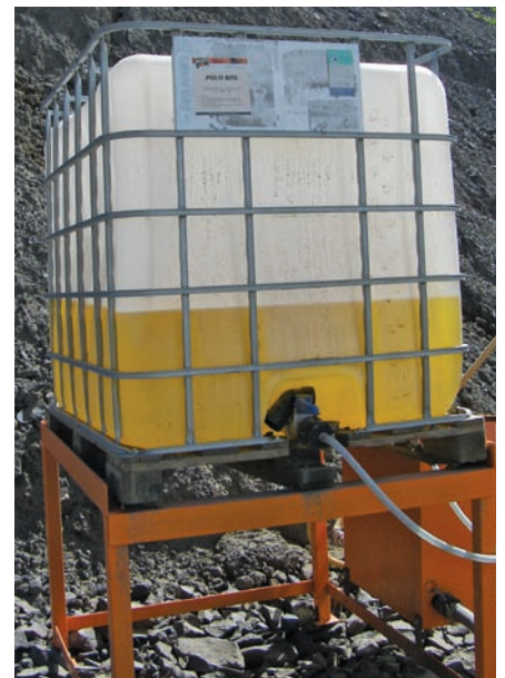
The 1000 litre container of the Polo BDS solution at Hi-Quality's Sunbury Quarry.
